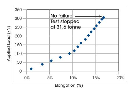
Break strength is the applied load at which the mooring line fails
