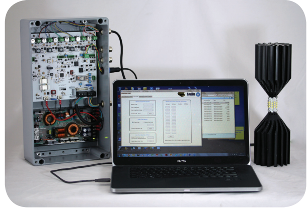
Shown with the Universal LED Controller, the light source is easily programmable using Sealite's PC Configuration Tool
