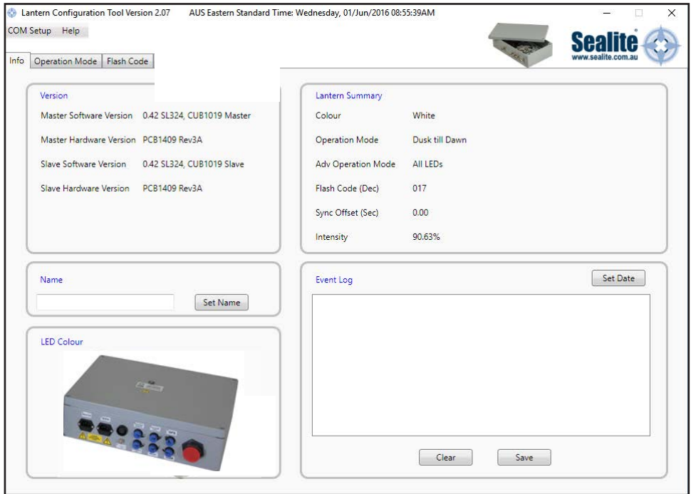
Image 3. Sealite Configuration Tool “Info” tab – showing COM Port connection established, Version & Lantern Summary information
