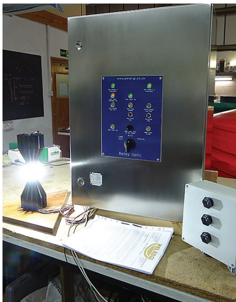
Front Panel of Control System to Commissioners of Irish lights specification driving the 78W 24V Light Source and combined Triple Photo cell
