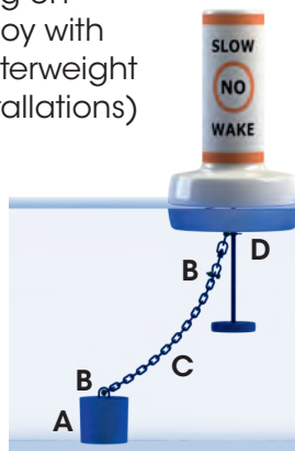
Shallow water chain mooring for float collar buoy
