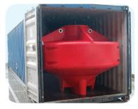
The hull section of the ATLANTIC-2600 has detachable side panels that are designed to be removed during transport, allowing the buoy to be conveniently transported in a shipping container. This provides the benefits of an extraordinarily large float section, without the need for a heavy, steel mooring-post.
